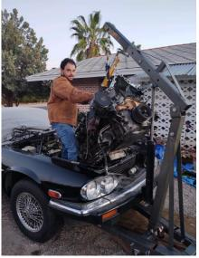
I got the non-running XJS running for a few quick days, with some new spark plugs, new injectors, some thrown wrenches, and very choice words. That was a win for around 2 days but then I soon realized, with thick smoke, oil shooting out from the exhaust. milk colored oil, and it over heating very quickly I had a
